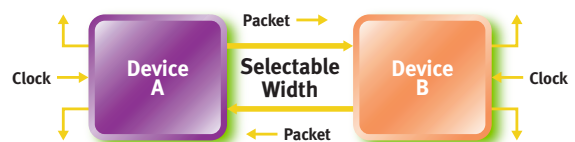
Figure 8. A 3GIO link uses transmit and receive signal pairs.
